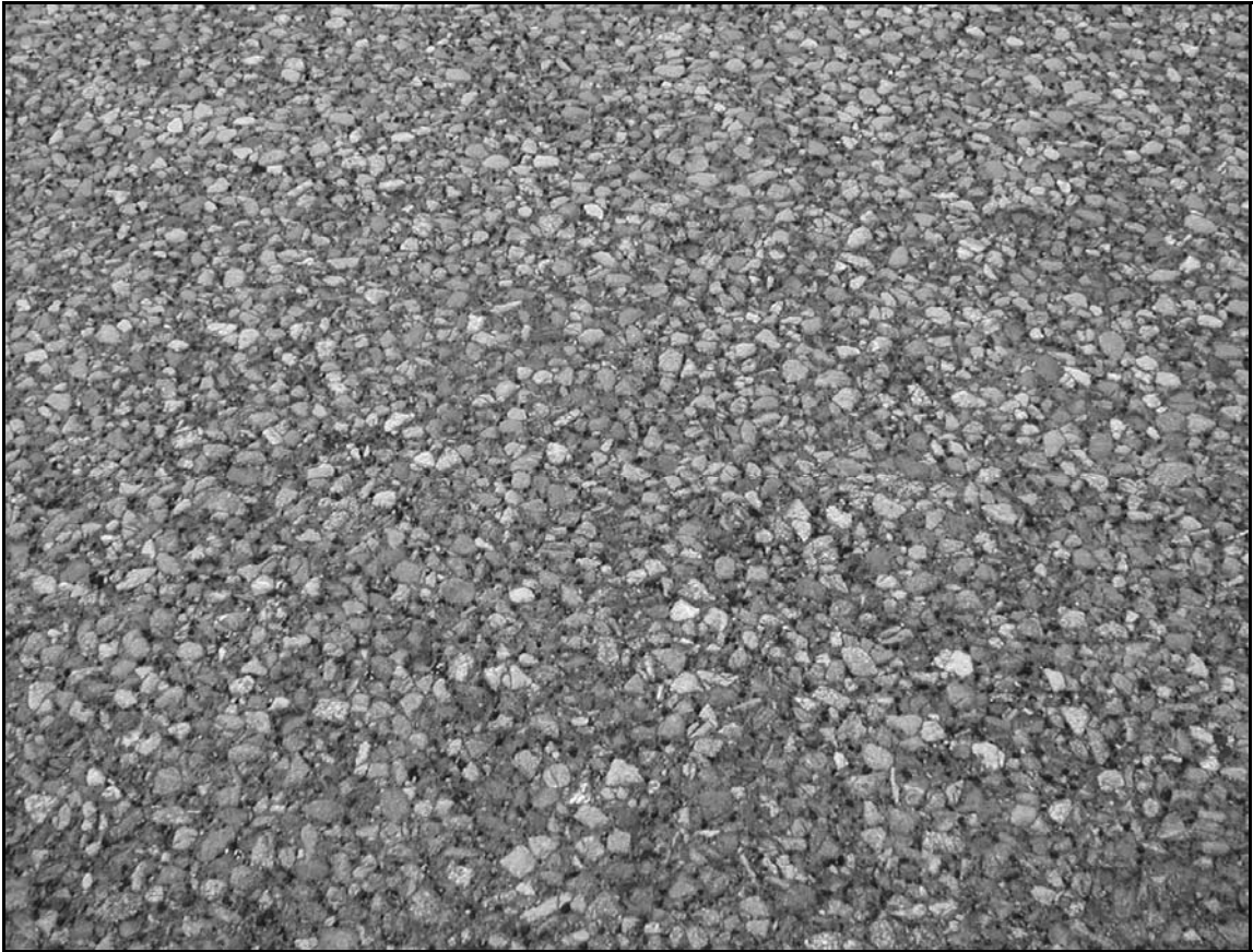
Photo 2.21: Close up photo of Anchorage Plus Ride Mix – note ground rubber pieces
