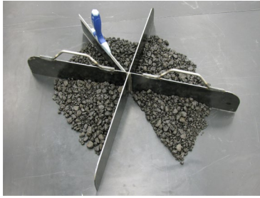
Asphalt mixture from the apex of the quarter to the outer edge.
