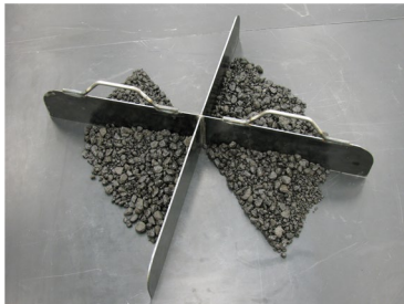
Equal portion from the diagonally opposite quarter
