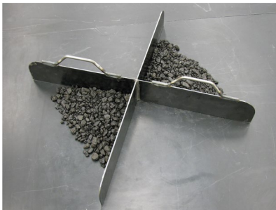
Diagonally opposite quarters removed
